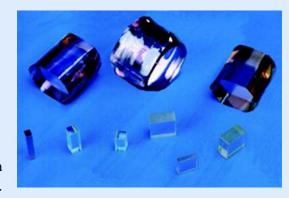
CASIX applies Czochralski (CZ) crystal growth technology to grow high grade Nd:YVO<sub>4</sub> crystals. With strict control of materials and the growth
