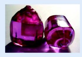
Nd:GdVO<sub>4</sub> crystals are excellent laser crystals. They are ideal laser host materials for diode pumped solid
