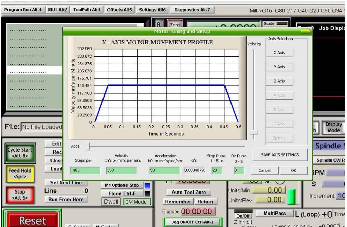
The setup is over, Please close the Mach software that all data setup can be available. And then open it again to check whether all the data is correct otherwise can't run your machine well.
