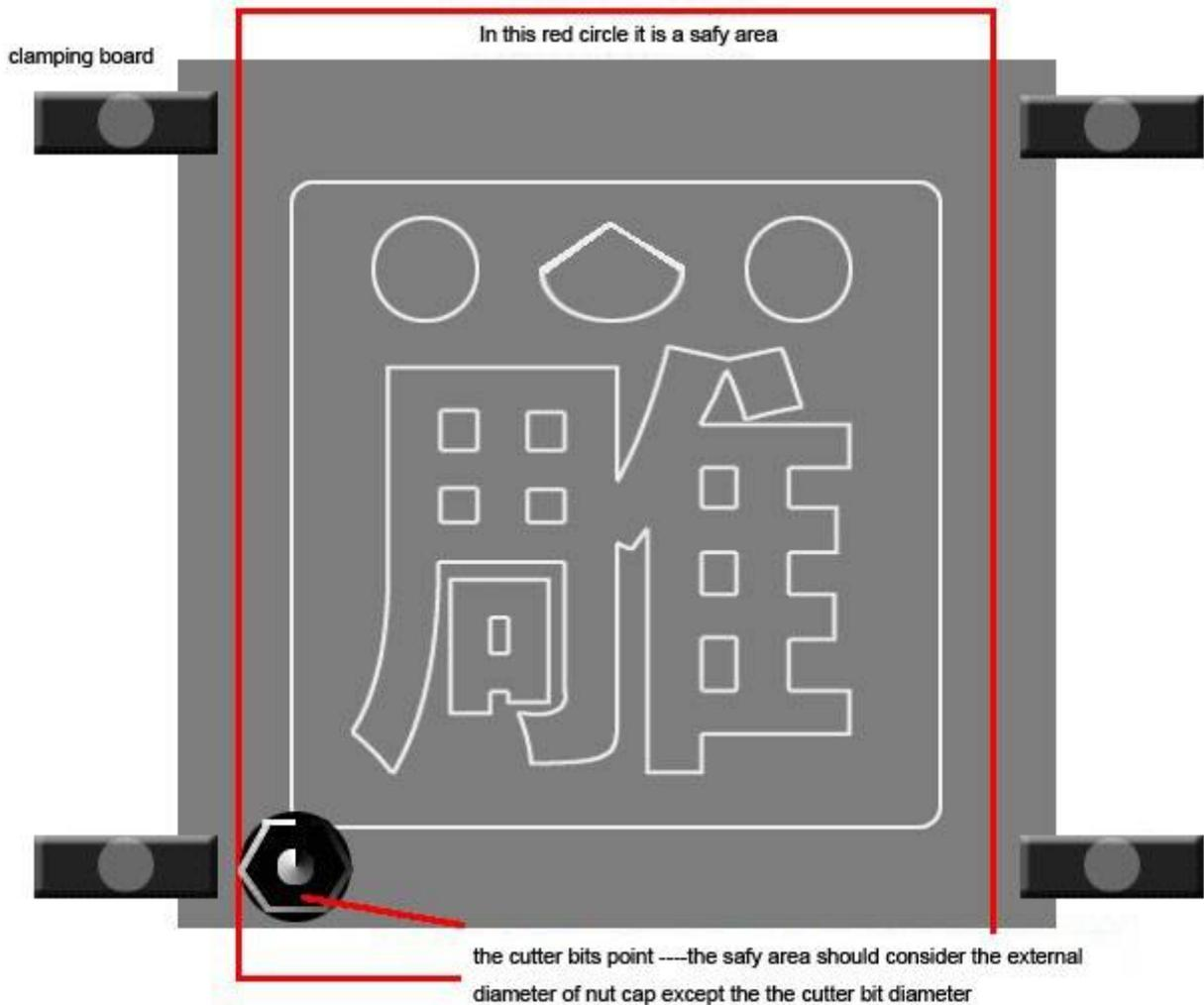
**Notice: when doing holed-out work, please put a no-use flat board below the material to avoid the damage of the working station**
