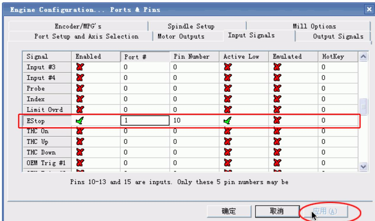
7. Limited Switch setting in “Ports and Pins” menu to click “Input Signals” and set X, Y, Z as below:
