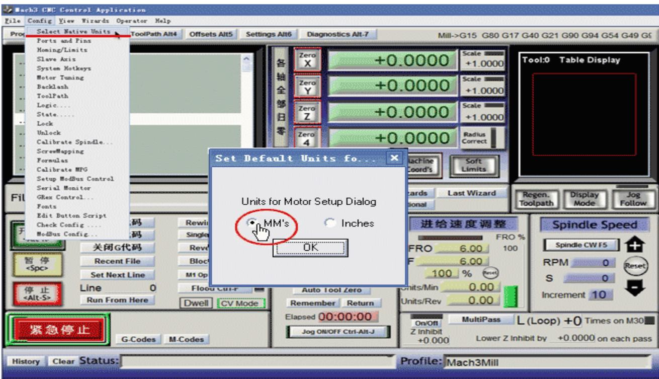
3. See as below, open "Config--Ports and Pins" to enter the setup.
