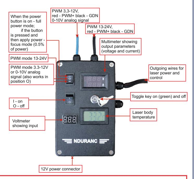
WARNING! PWM duty cycle should not exceed 99%. Unused wire of PWM to reduce interference need to twist at the end (black with red)
