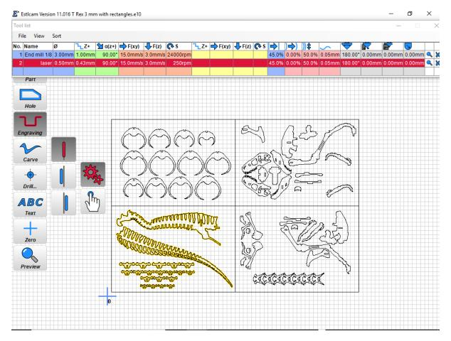
My tool path depth is set at 3.4mm and my Laser Depth per Pass is set at 0.43, which will work out at 8 passes per object dropping my Z Axis height 0.43 mm each pass.
