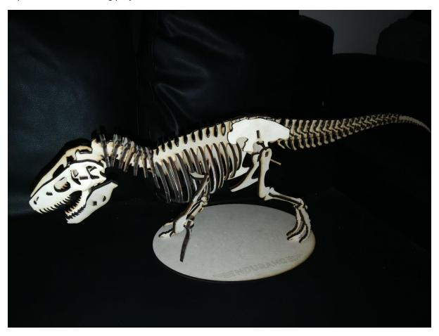
Please note that I like the surface discolouration of the wood, makes it more aged and bone like, but to prevent this I found blue painters tape stuck to the work surface removes the surface discolouration.
