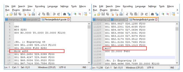
So for each engraving I insert my Laser Start and End Codes, for me using Marlin and Ramps 1.4 my Laser On is Code M106 S\*\*\* \*\*\* represents the power to the laser 0 = off, 255 = full power and Laser Off Code is M107. Please see above, these codes are placed at the start and beginning of each Engraving Pattern.
