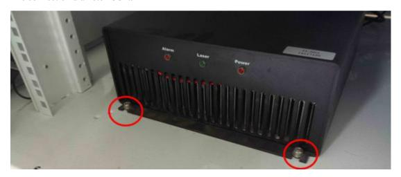
Using four fixed holes on the laser to fixed the power supply into right place.
