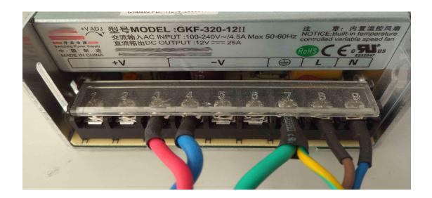
D: Power supply connected to the laser control card, for the modulation signal is used to control the laser output.
