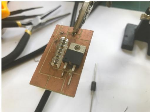
Be sure to use enough solder to create a thermal connection – the 13N10 dissipates a lot of heat to the PCB. Insufficient solder will result in overheating of the MOSFET.
