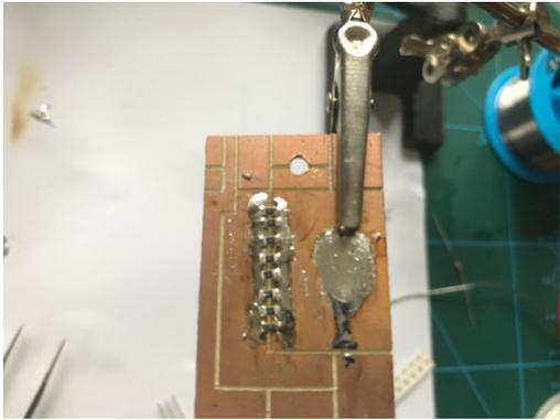
The centre connector on the 13N10 is not needed – ground is completed through the back plate soldered to the PCB. Trim it off, then solder the 13N10 to the PCB
