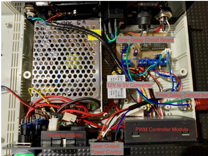
After proving the prototyped delay circuit I made engraved a PCB to make a much nicer final version. CCT diagram at the end of this document.
